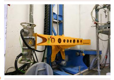
Following the same operation principles, macrotomographic acquisitions can be realized on larger-sized pieces up to 40 cm by side. In this case, the scan is realized on a custom-built Macrotom operating at 420 kV, with a minimum pixel size of 360 µm. A specific acquisition procedure, data processing and reporting will be provided according to the demand.
